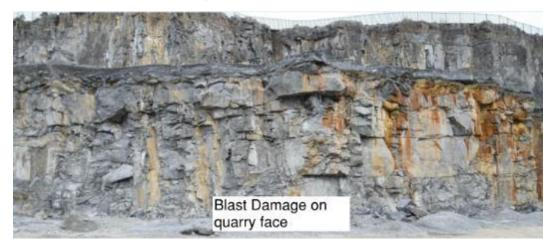
Figure 3.17: Blast damage on quarry face
